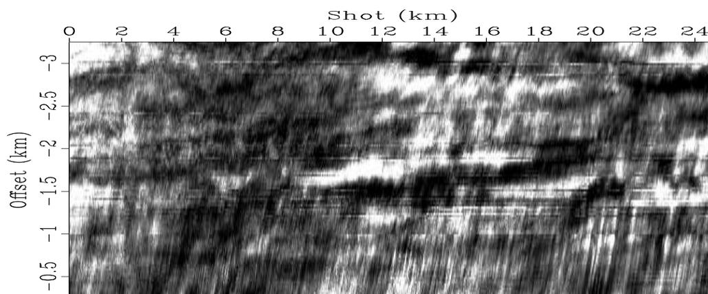
Figure 12: 2-D amplitude map corrected for variations in the source, offset, and receiver directions using the coefficient curves in Figures 4, 5, and 7.
