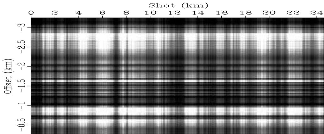
Figure 8: Synthetic 2-D amplitude map modeled using the source and offset coefficients.
