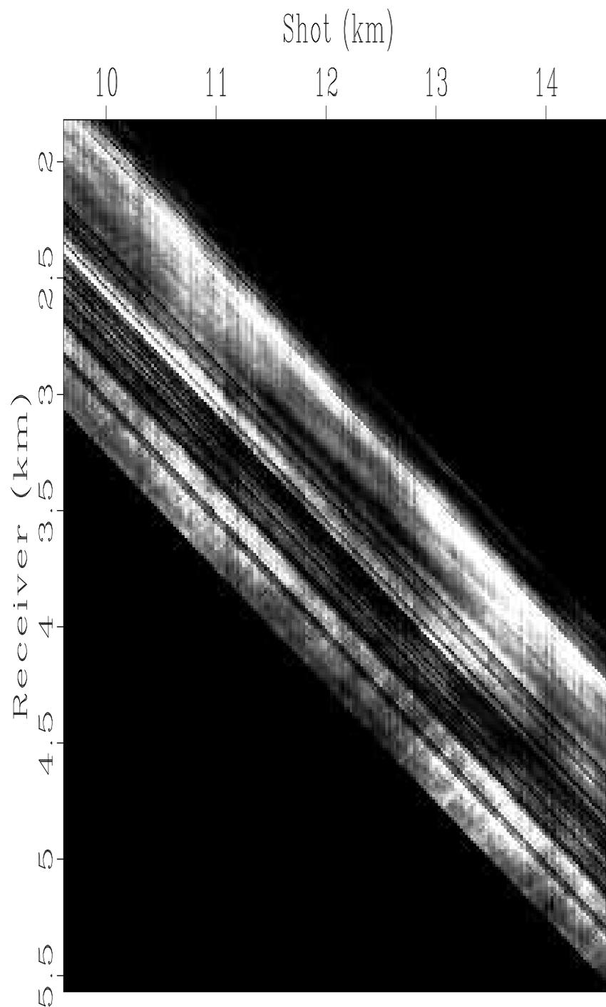
Figure 3: Portion of the amplitude map in Figure 1 displayed in the source and receiver space. The stripes along the descending diagonal follow the offset direction. Midpoint and receiver stripes are less visible in this coordinate system.
