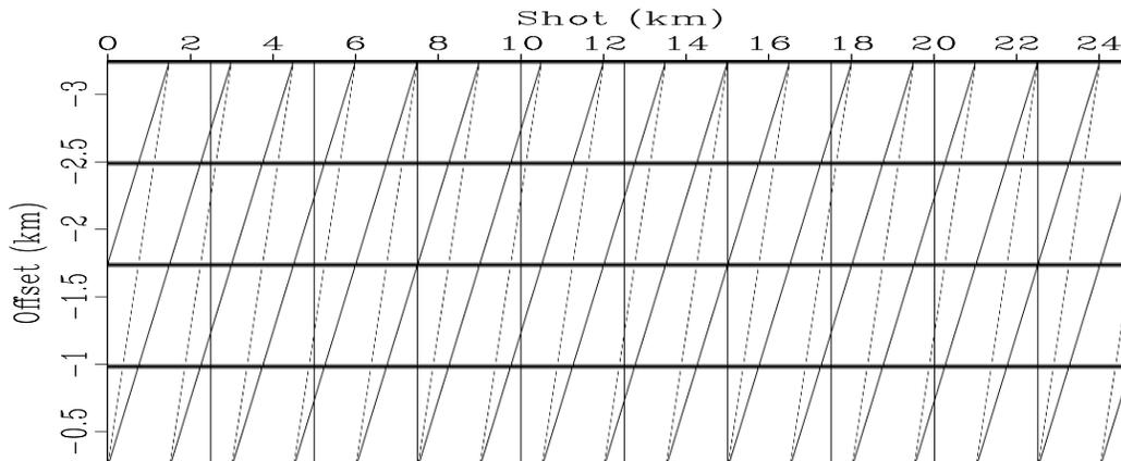
Figure 2: Model of offset-, source-, midpoint-, and receiver-consistent stripes, based on the 2-D amplitude plot in Figure 1. The solid dipping lines correspond to the receiver-consistent stripes, and the dotted lines represent the midpoint-consistent stripes.
