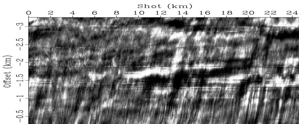
Figure 9: 2-D amplitude map corrected for variations in the source and offset directions using the coefficient curves in Figures 4 and 5.
