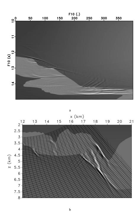
Figure 6: Migrated images using wavefield extrapolation in Riemannian coordinates with a Fourier finite-differences (F15) kernel. Panel (a) depicts the image in Riemannian coordinates, and panel (b) depicts the same image mapped to vertical Cartesian coordinates.
