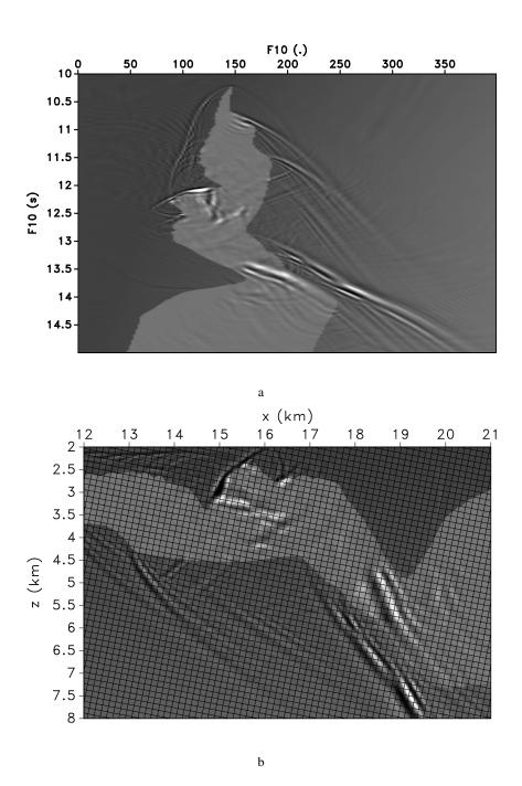
Figure 7: Migrated images using wavefield extrapolation in tilted Cartesian coordinates with a Fourier finite-differences (F15) kernel. Panel (a) depicts the image in tilted Cartesian coordinates, and panel (b) depicts the same image mapped to vertical Cartesian coordinates.
